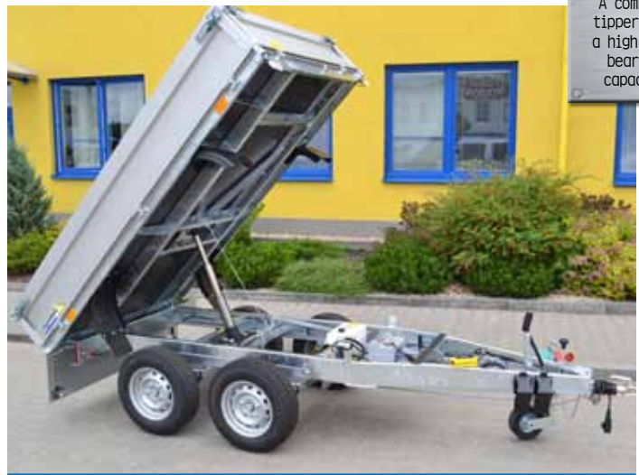
DELTA Trailer with manual (electrical) control of the hydraulic system
