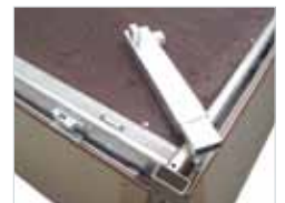
Anchoring yokes in the side bar of the trailer
