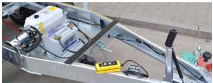
Electrical control of the hydraulic system with a removable controller
