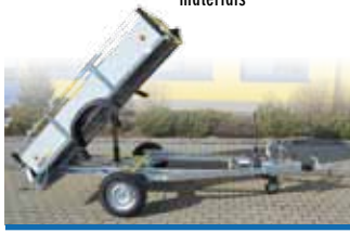
Trailer VZ 26 with a hydraulically tilting body
