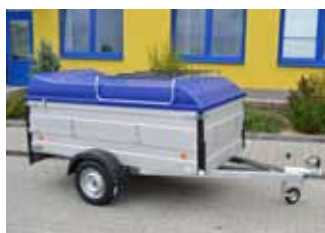
ALUX 26 N1 with an extension of 350 mm and a laminated cover
