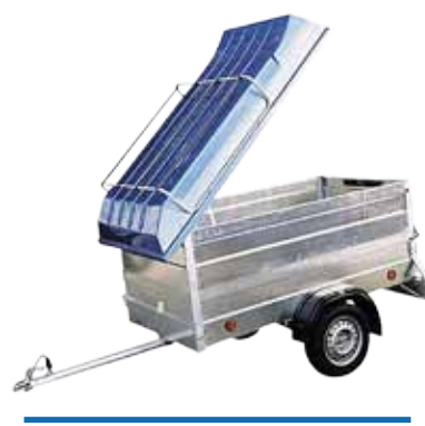
Trailer NP 3 with side board extensions and a lockable cover
