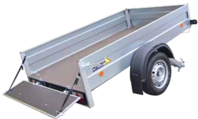
Trailer HANDY 8 in a tilting variant with reinforced rear board as the ramp
