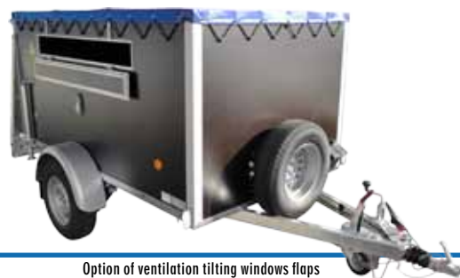
Option of ventilation tilting windows flaps
