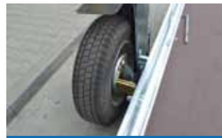
Hydraulically tilting axle
