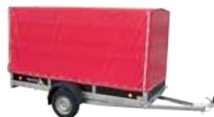
Unbraked trailer VZ 30 with canvas and a construction with the loading height 1.92 m
