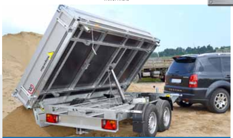
All-welded upper and lower frame with a high-performance hydraulic system
