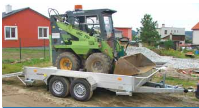
Aluminium transport trailer for excavators
