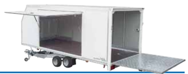
Trailer ADAM with an aluminium box in the design for transport of cars
