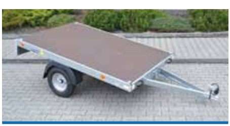
TITUS trailer in the plateau design with 10" wheels
