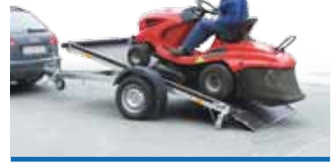
Trailer VZ 26 N1 750 kg, tilting platform
