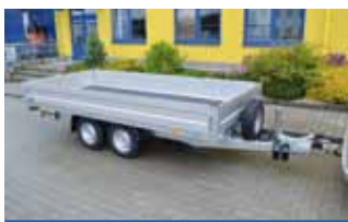
Trailer with rear supporting legs and a spare wheel
