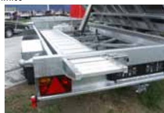
Aluminium access parts can be easily stored in the lower frame
