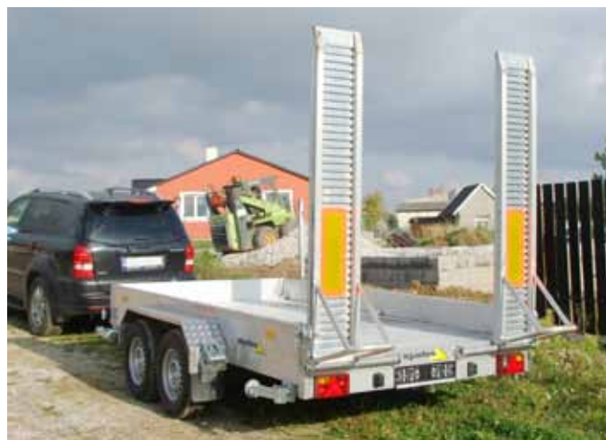
Rear integrated aluminium loading ramps
