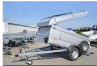
Tilting braked trailer VZ 26 with aluminium side boards, with a spare wheel, extension of side boards and a laminated cover
