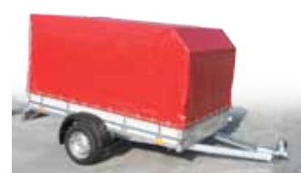
Option of extension of side boards and canvas with a construction for the KANGAROO type
