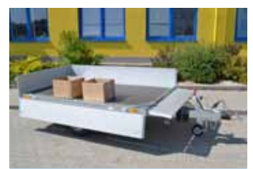
Easy tilting of aluminium side boards
