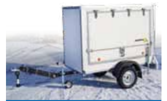
Trailer with a side flap and height-adjustable drawbar
