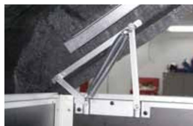
Simple system of attachment and tilting function of the cover
