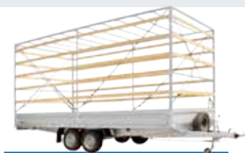
Solid canvas construction with removable upper cross - bars
