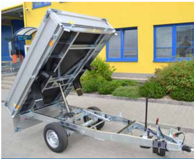
Trailer DELTA B2 with electrical control of the hydraulic system
