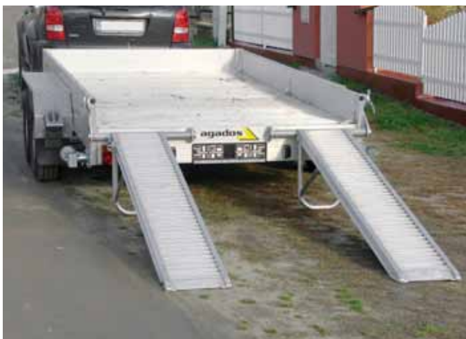
Rear integrated aluminium loading ramps
