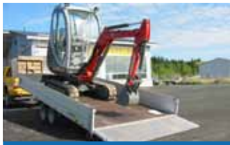
Platform design with a drive-up ramp
