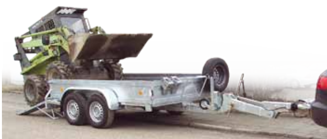
Trailer S1 with a height-adjustable drawbar and a possibility of replacement of the DIN 40 drawbar lug with the ISO 50 coupling
