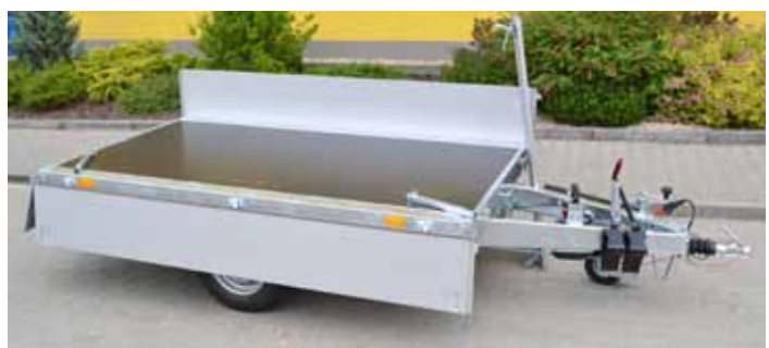
Easy tilting and removal of side boards and a posts
