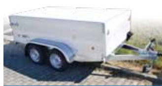
Trailer with increased aluminium side boards and an aluminium cover
