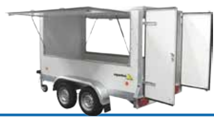
Trailer with side flaps and rear double-wing door
