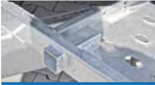
Preparation for the winch
