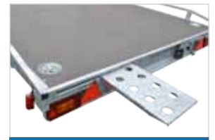
Removable access parts and anchoring eyes folding in the floor
